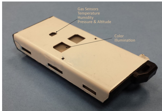
Fig. 3. Sensordrone device with different sensors (ambient temperature, precision gas, humidity and altitude are utilized in this paper). Device dimensions: 2.67 x 1.10 x 0.49 inch 3 .
